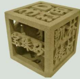
Sand Core Made By 3D Printing
