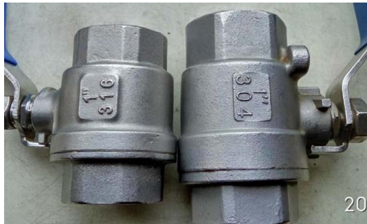
Fig.12 Component by ceramic sand shell method (left) and by investment process (right)
