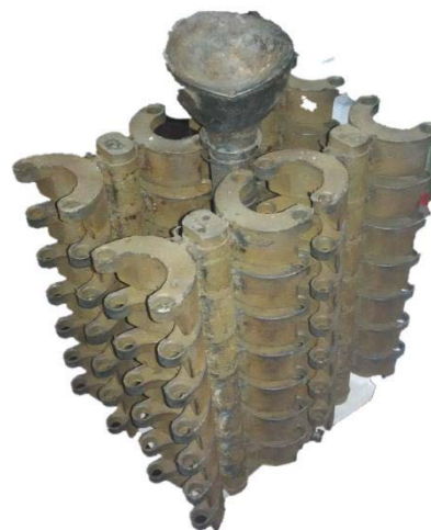
Fig.3 Components clutch with gating system after casting
