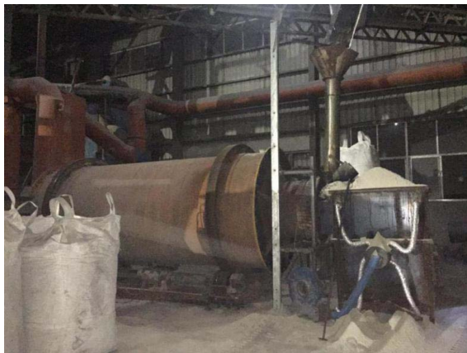
Fig.16 A sand reclamation rotary drum (gas fueled)
