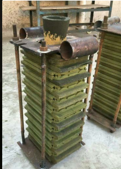
Fig.5 Shell method cores assembled to cast
