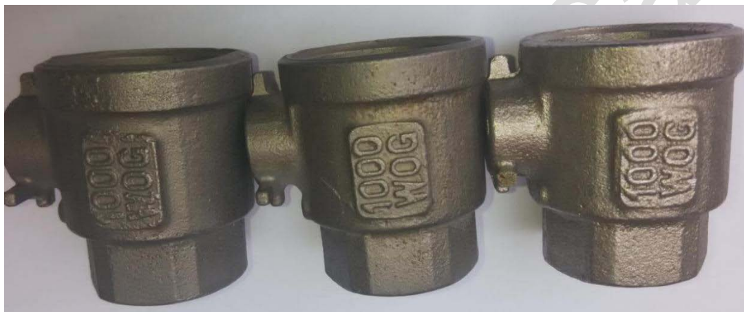
Fig.13 Castings of ceramic sand shell method after drum shot blasting
