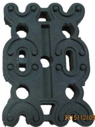
Fig.2 Shell method sand core
