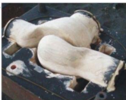
Figure 3 Wuxi KOSO Valve using Kailin Ceramic Foundry Sand molding core
