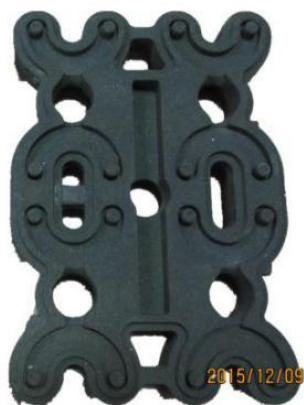
(a) Single core piece for shell method
