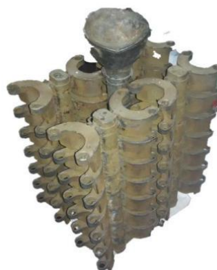
(b) Castings clutch with gating system made by shell method
