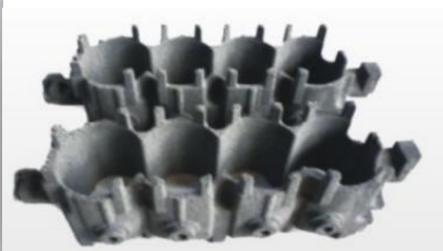
(b) Water jacket core of cylinder block
