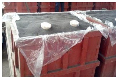
(b) Molding by using ceramic sand
