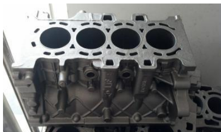
(c) A cylinder block made by lost foam process
