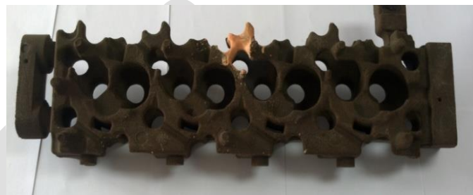
(a) Water jacket core of cylinder head
