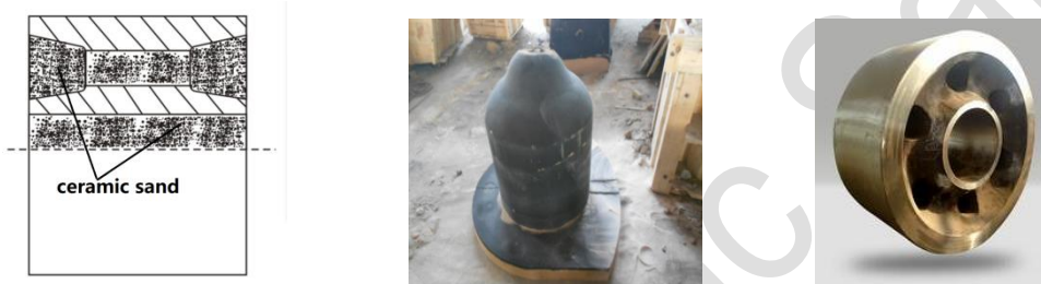
(a) Filling position of ceramic sand (b) Ceramic sand using at core surface (c) Supporting roller (cast steel)
