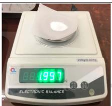
Weigh 0.5000g of grinded sand samples (accuracy; 0.0001g), put into the reagent solution.
