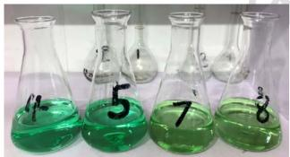
10 (Determining the content of iron oxide) Add 10ml of testing solution into a volumetric flask of 100m, add water to a volume of 50ml.
