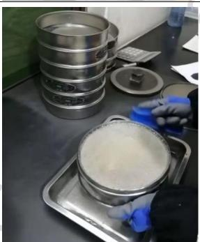
7. Place the sand in each tray on an electronic scale and weight it
