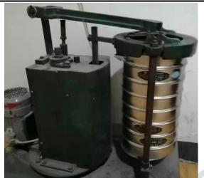
Remove the sieving dish and place the sieved samples in the corresponding tray
