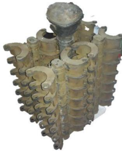
Castings clutch with gating system made by shell method
