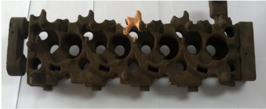
Water jacket sand core of cylinder head made by Kailin ceramic sand RCS
