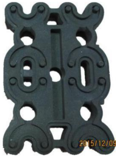
Single core piece for shell method (ceramic sand RCS)
