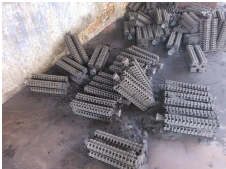
Single core piece for shell method (ceramic sand RCS)
