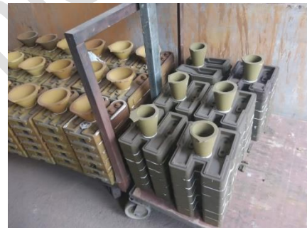
Castings clutch with gating system made by shell method
